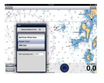
" he WLN10 also works well with the populat iNavX charting program. Choose the WLN10HS for AIS based systems as this is preprogrammed in the factory for 38400 baud NMEA data. Of course, you can reconfigure in the field but its nice to plug 'n' play straight out of the box"
