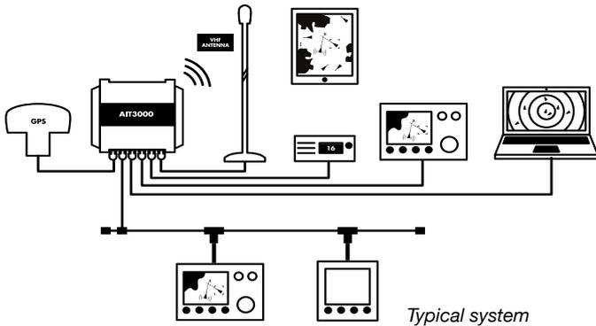
The AIT3000 offers multiple interfaces allowing connectivity with any AIS ready plotter. Choose from NMEA0183, NMEA2000 and USB (for PC and MAC). There's also a built in WiFi server to send data over a WiFi link to iPads, iPhones or tablets and a host of supported apps and navigation programs.
