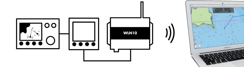
This is the preferred solution as it allows a cable free and easy installation.
