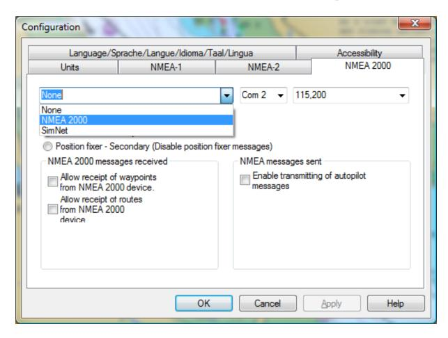
In addition to dual NMEA 0183 interfaces, SmarterTrack can also connect to a NMEA 2000 system via Digital Yacht's NMEA 2000 USB gateway
