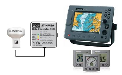
NMEA sensors like the GPS150 can connect to the ST interface and provide an output to the SeaTalk bus
