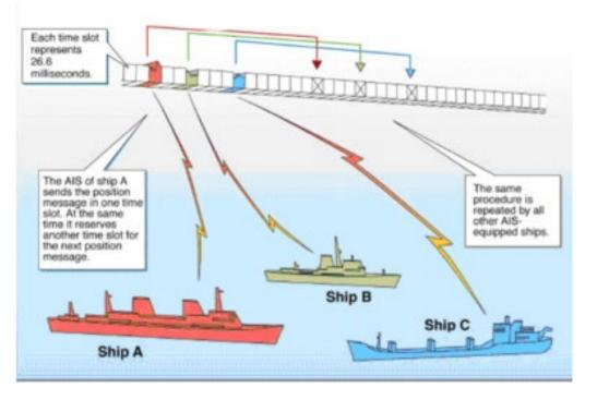
Class B+ is a new generation of AIS functionality based on SOTDMA (self organised TMDA) messaging rather than the simpler CSTDMA (carrier sense TDMA). It guarantees your AIS transmission will get a time slot, even in areas of very high traffic density.
