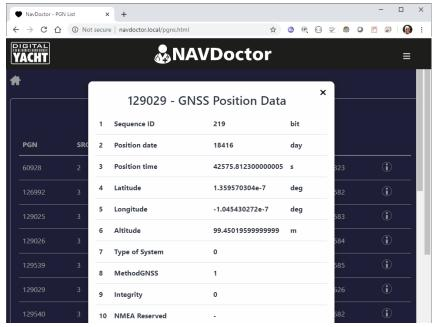
PGN list shows all data PGNs on network (including source and destination) with drill down and decoding
