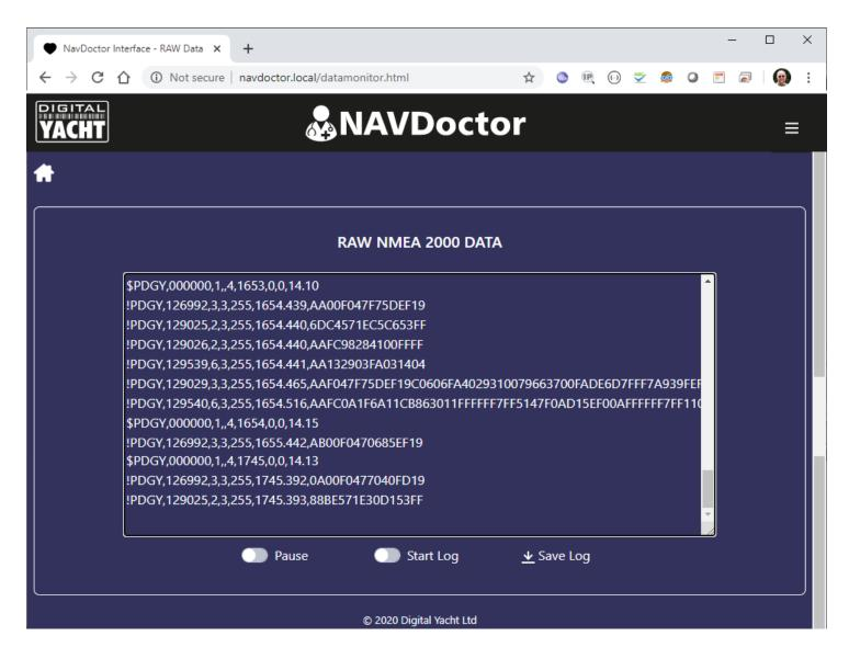
Raw data log allows logging and saving of data for analysis (as a simple text file) as well as the ability to pause data display
