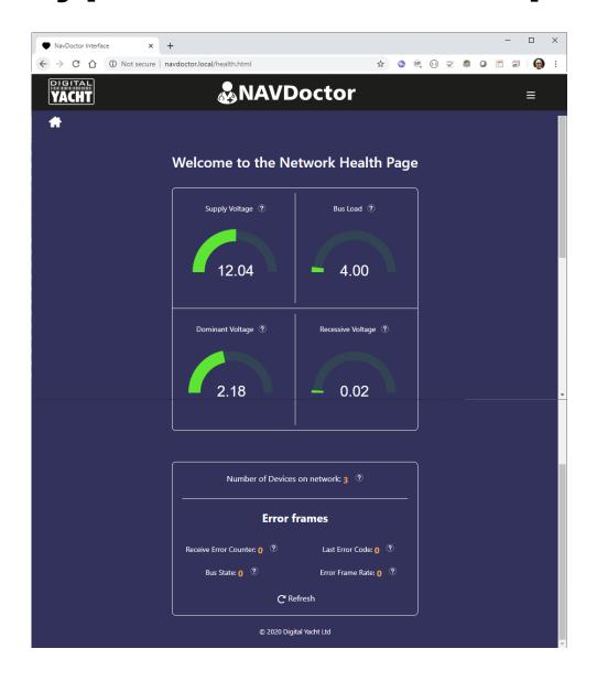
NAVDoctor also checks the physical status of the network and shows supply voltage, bus load, dominant and recessive voltage and error frame rate
