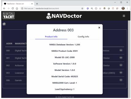
Device list shows all devices on the network with drill down providing extended information such as serial number, software version and NMEA certification and product ID
