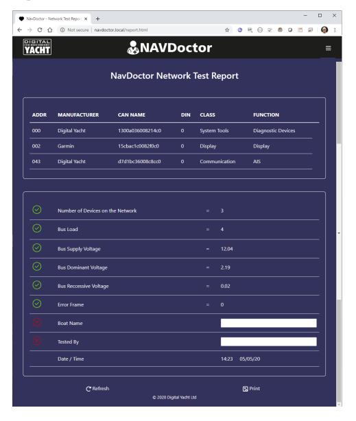
NAVDoctor can generate a printable network summary test report which is ideal for technicians to offer customers as a validation of the installation.
