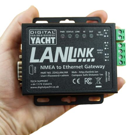
LANLink is available in two versions suitable for NMEA 0183 and NMEA 2000 respectively. It features an easy to use web interface allowing any device with a browser to configure NMEA baud rates and IP/Port information.
