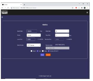
Configure NMEA data for 4800 or 38400 baud and set mode (TCP/IP or UDP) and port
