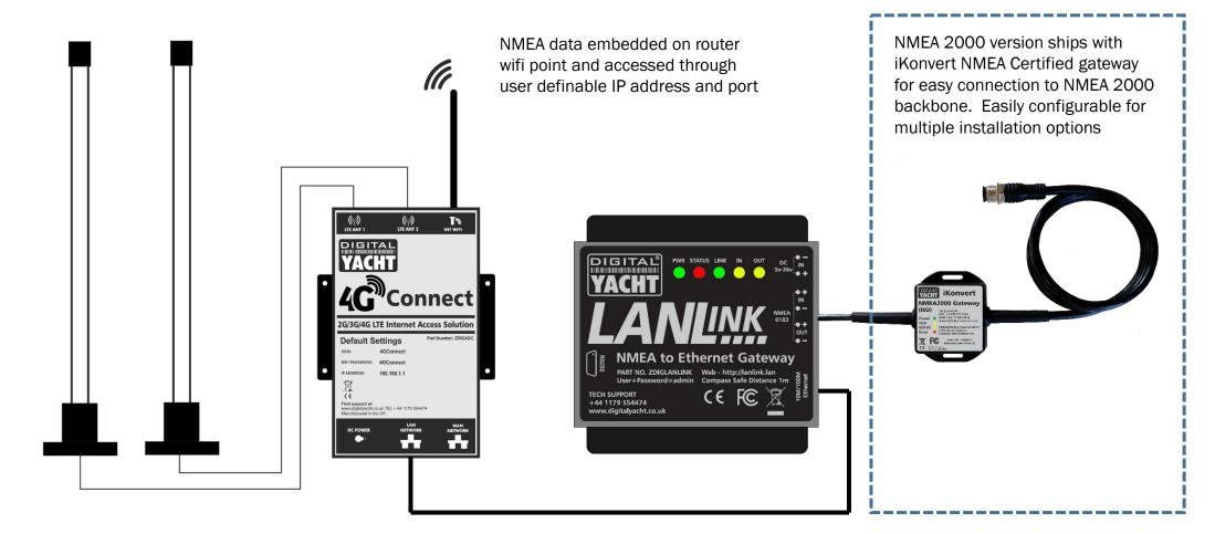
Simple ethernet patch cable connection to router
