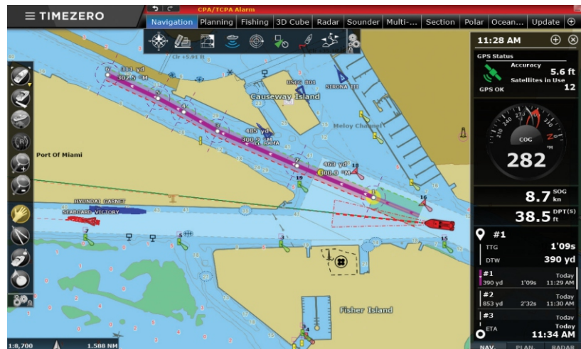
Advanced AIS displays with CPA and TCPA alarms
