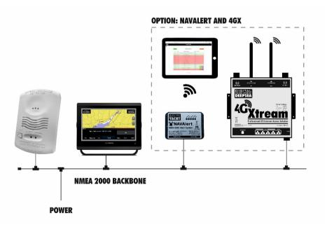
CO Alert creates a standard NMEA 2000 alert PGN which allows pop up alarms on compatible MFDs. (At present, this functionality is best implemented by Garmin)
