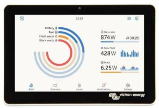
Wireless interface for tablet and iPad setup, monitoring and internet gateway connectivity
