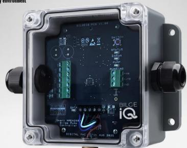
Full NMEA 2000 integration with MFD control and industry standard NMEA 2000 alerts Wireless interface for tablet and iPad setup, monitoring and control. Can also join an existing on board wifi network
