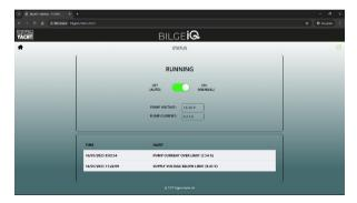
Control the pump from wireless display, manual switch or MFD. Curent consumption of pump indicated in real time to show correct operation
